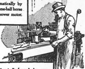
Electrically-heated glue-pots are used in pattern shops and elsewhere.
